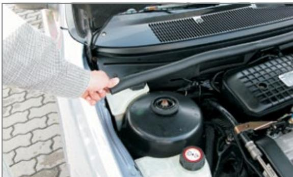
**EN** Remove the rubber seal
