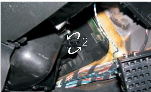
(EN) Loosen the screw on the cover, turn the lock 90 degrees to the left and remove the filter cover
