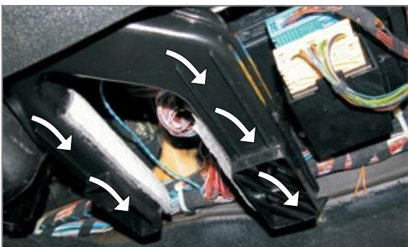
(EN) Disassemble the segment of the ventilation collector pipe and remove the collector
