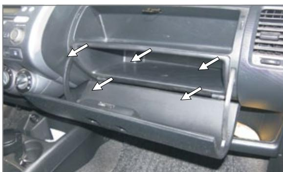
**(EN)** Remove the glove compartment
