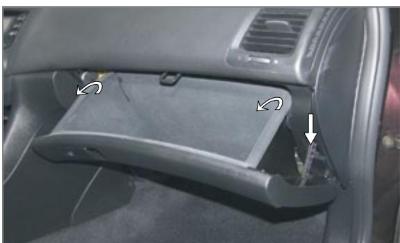
**EN** Remove the glove compartment
